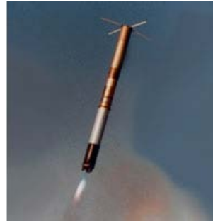
MK 234 Electronic Decoy Cartridge (Nulka)
