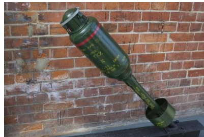
Anti-submarine charge (hedgehog) Length 100 cm Diameter 18 cm
